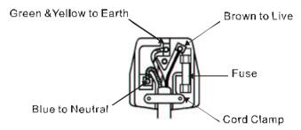
The wire which is coloured GREEN and YELLOW must be connected to the terminal in the plug which is marked with the letter E or by the earth symbol ④ or coloured GREEN or GREEN and YELLOW.
